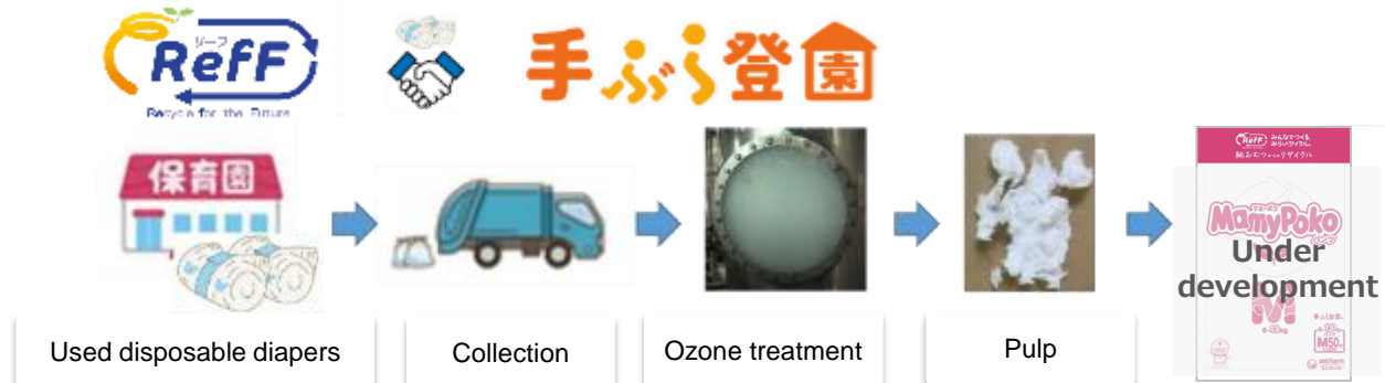
Flow of collecting used disposable diapers from nursery school facilities and recycling them
